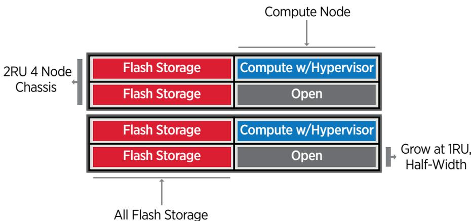
Figure 1) NetApp HCI Minimum Configuration
